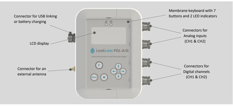
The main components of the device are:
